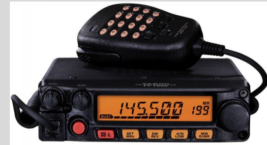
VHF Radio Station
