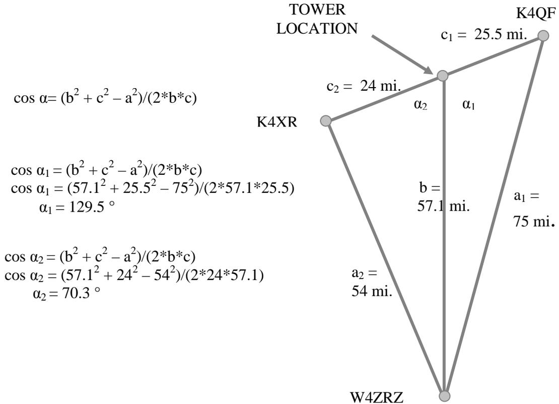
**Figure 5 - Geometry For Tower Contacts**
