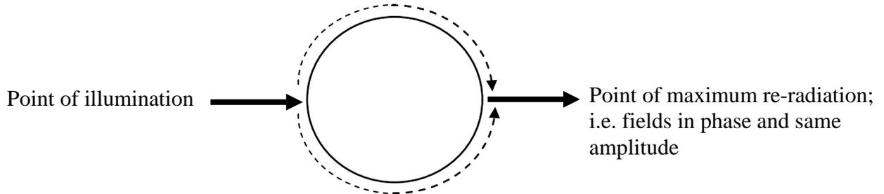
**Figure 7 - Surface Current Distribution Around A Sphere**
