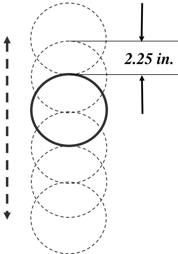
**Figure 8 - Tower Leg Generation From Sphere Stacking**
