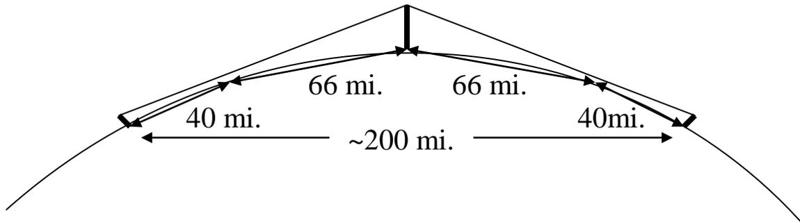
**Figure 2 - TV Transmitting Tower Geometry For Typical Contacts**
