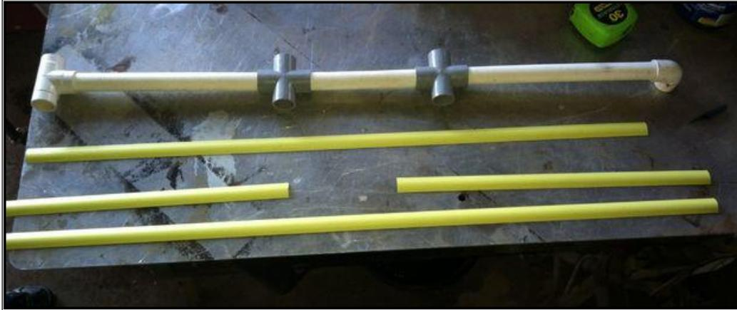
You'll need to cut two pieces of PVC pipe. One piece will be **11 1/2"**, the other **7"**. This, along with the PVC connectors, will form the frame of the antenna.
